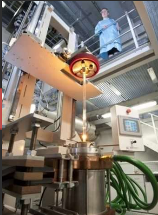
(Fiber drawing tower, ORC, Univ. of Southampton)
